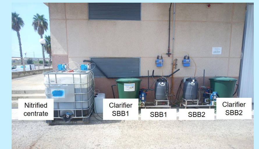
Fig. 2 – Biodesulphurisation pilot plant.
